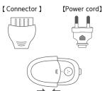
$\bigstar$  Please connect the connector fully as shown in the diagram
